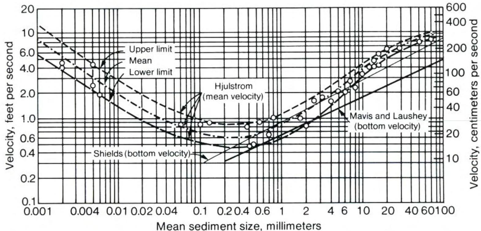
Critical water velocities for quartz sediment as function of mean grain size (after ASCE Task Committee, 1967).
