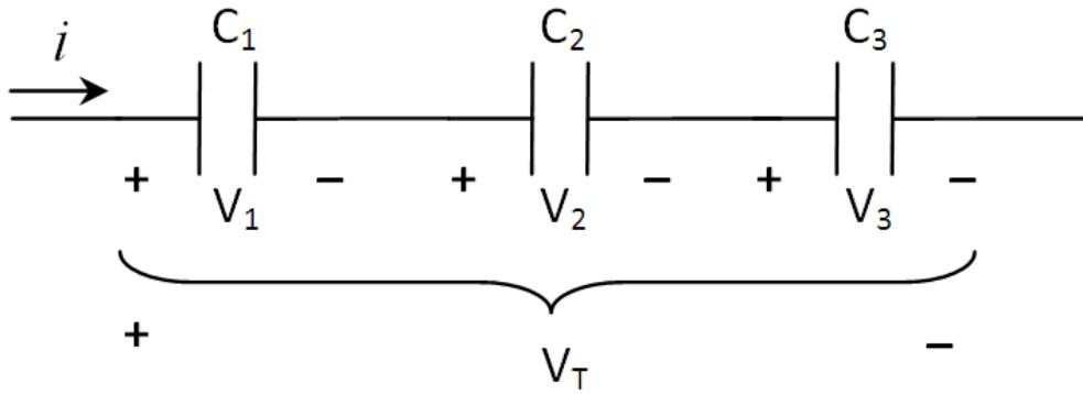
$$V_T = V_1 + V_2 + V_3$$
