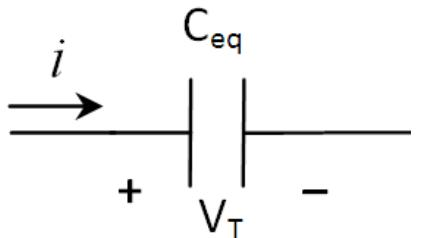
$$\frac{1}{C_{eq}} = \frac{1}{C_1} + \frac{1}{C_2} + \frac{1}{C_3}$$
