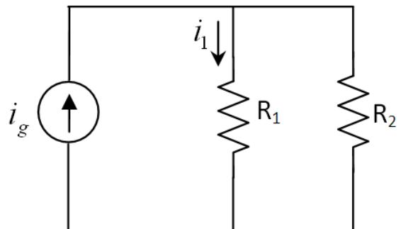
$$i_1 = i_g \frac{\frac{1}{R_1}}{\frac{1}{R_1} + \frac{1}{R_2}} = \frac{\frac{1}{R_1}}{\frac{R_1 + R_2}{R_1 R_2}} = \frac{R_2}{R_1 + R_2}$$
