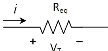
$$R_{eq} = R_1 + R_2 + R_3$$
