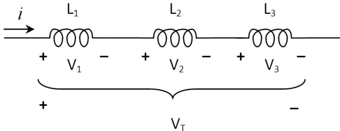
$$V_T = V_1 + V_2 + V_3$$
