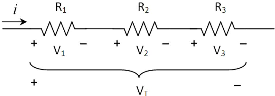
$$V_T = V_1 + V_2 + V_3$$
