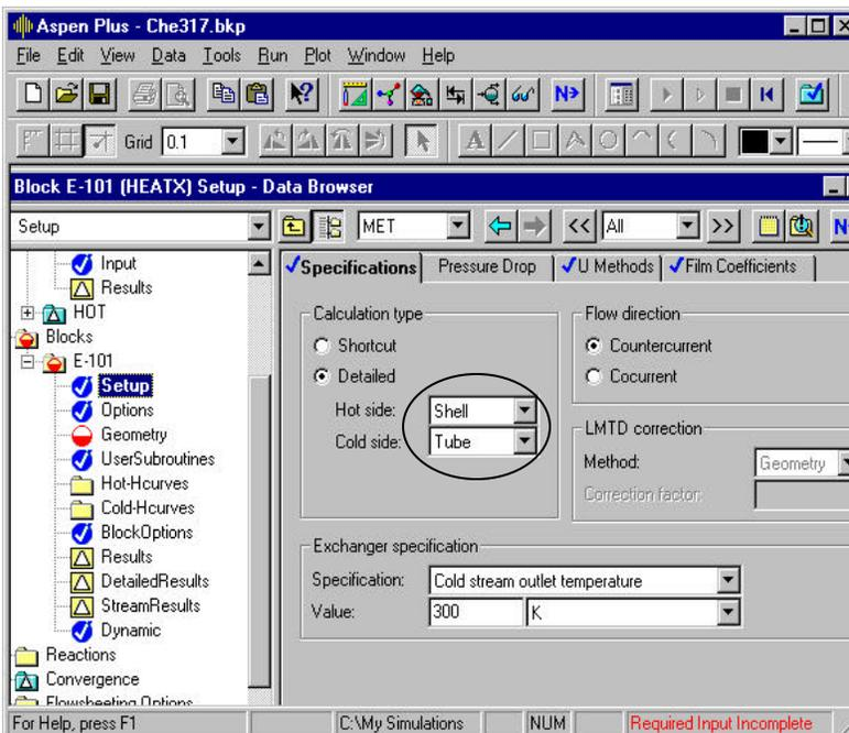
The **Setup** page is shown at left. First of all, change the calculation type from shortcut to the detailed method. Immediately, Aspen will ask you to identify which fluid goes where, shell or tube? For this example, use what is entered in the picture. In addition, Aspen will now calculate a LMTD correction for the exchanger. The default setting is the correction based on the geometry and that will be fine.
