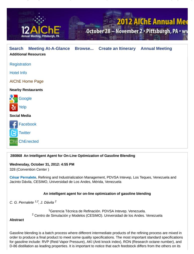
properties and cost. Therefore, in order to reach a finished product that respects the aforementioned constraints and using the available volume of each feedstock, an optimization problem must be resolved, normally off-line, that is, previously and without intervention in the actual blending process in real time.
