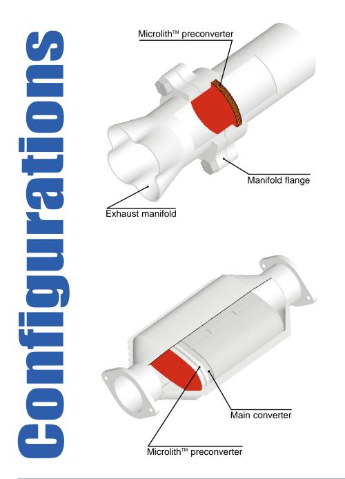
The small size of the coated metallic substrate allows design flexibility in positioning and mounting the preconverter.
