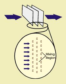
Mass Transfer Coefficient The short channel length and the higher geometric surface area of the Microlith<sup>™</sup> allows a 10 fold increase in catalystpollutant interaction.
