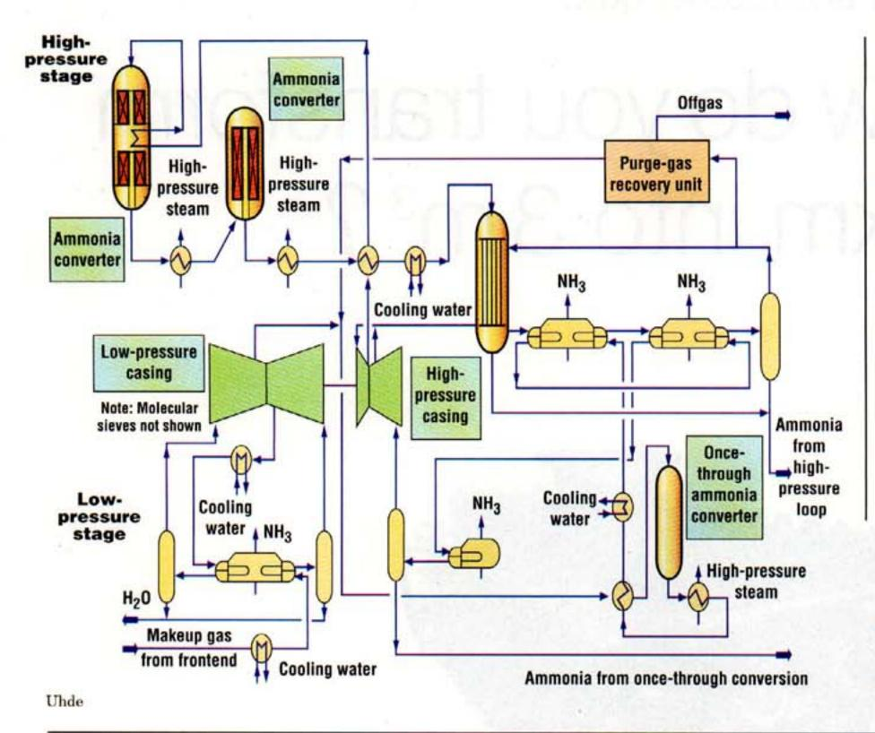
be conducted at 90 bars instead of the normal pressure of around 200 bars, thereby lowering capital and energy costs. Magnetite is used in the first bed of the synthesis loop, when the ammonia concentration is below 2% of the feed, then ruthenium is used in the next three beds to bring the ammonia level up to 18% or more.
