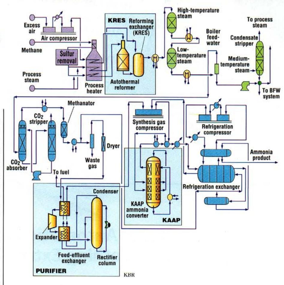
For ammonia synthesis using the KAAP process, a ruthenium catalyst (on a carbon support) is used in three of four beds. Reaction to be conducted at 90 bars instead of the normal pressure of about 200 bars for a standard magnetite catalyst
