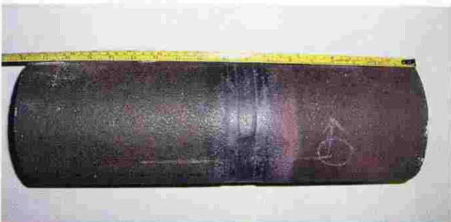
FIG. 3. No cracks were observed in riser B.
