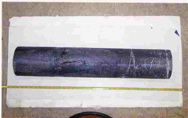
FIG. 1. A longitudinal crack developed in riser A.
