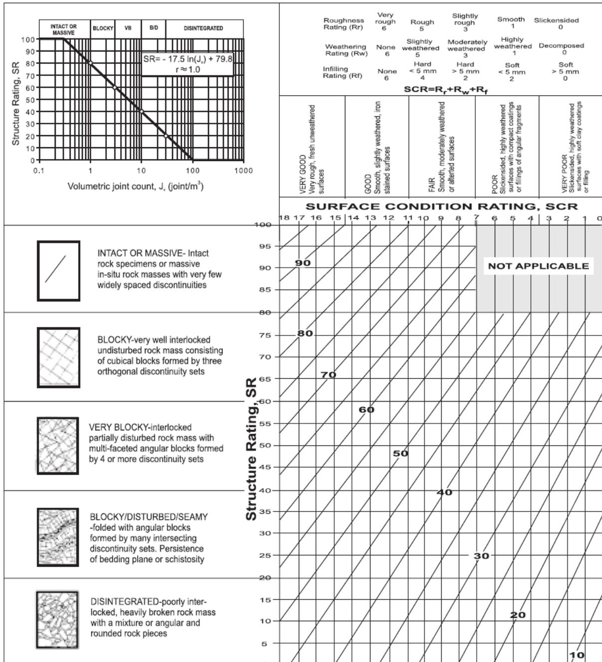
Figure 6. The modified quantitative GSI System suggested in this study.
