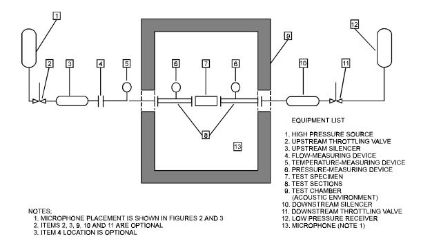
Figure 1 — Control valve noise test — system components
