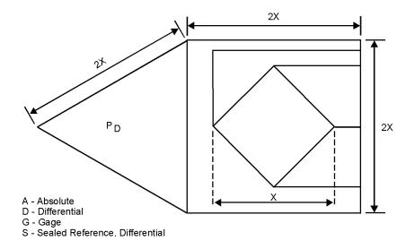
The strain gage is symbolized by a small square, with diagonals x by x, centered in the large square. The diagonals of the small square are drawn perpendicular to the sides of the large squares. Lines from each apex of the small square projected to the right side of the large square represent the electrical leads.
