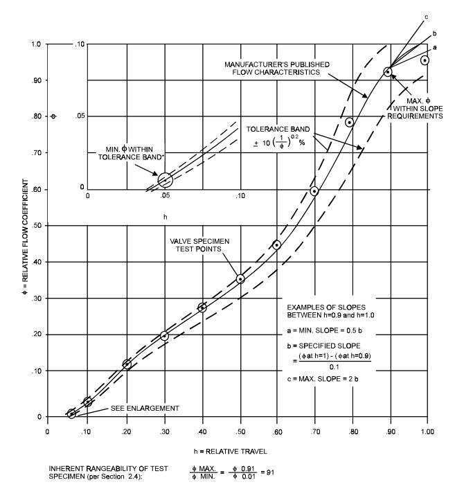
The maximum flow coefficient  $\phi$  meeting the requirements of Section 4 is 0.91; the minimum  $\phi$  is 0.01.
