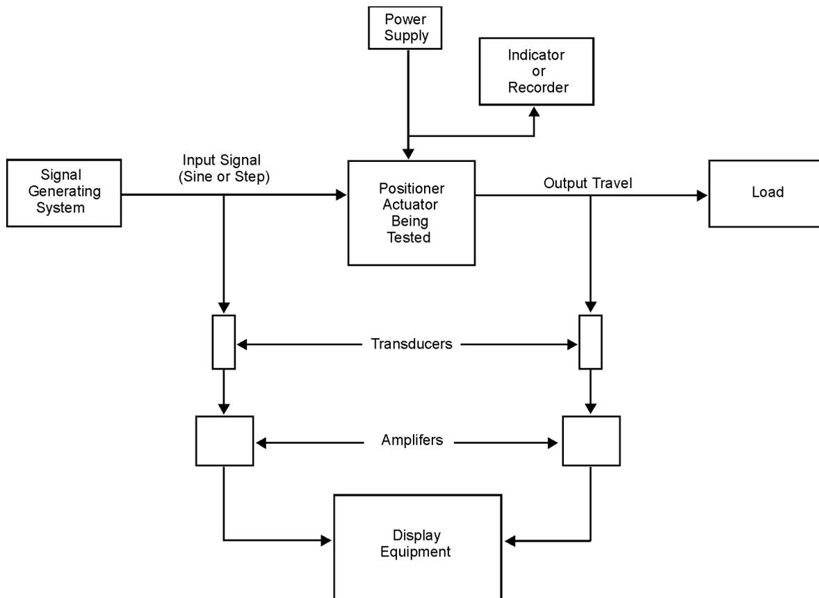
Figure 12 — Schematic of simple dynamic response test system
