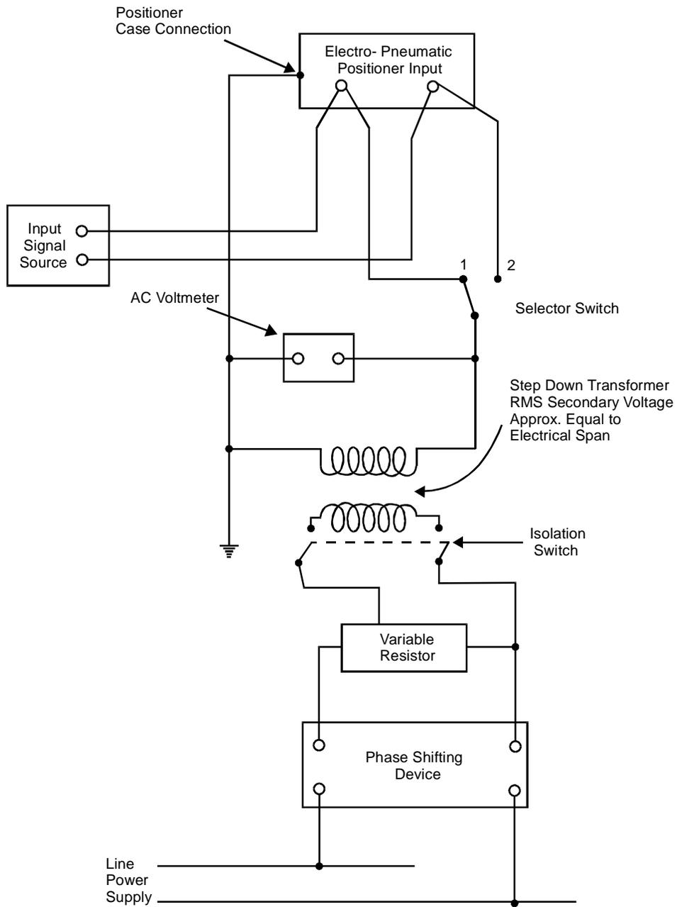
**Figure 7 — Test circuit for common mode interference influence**
