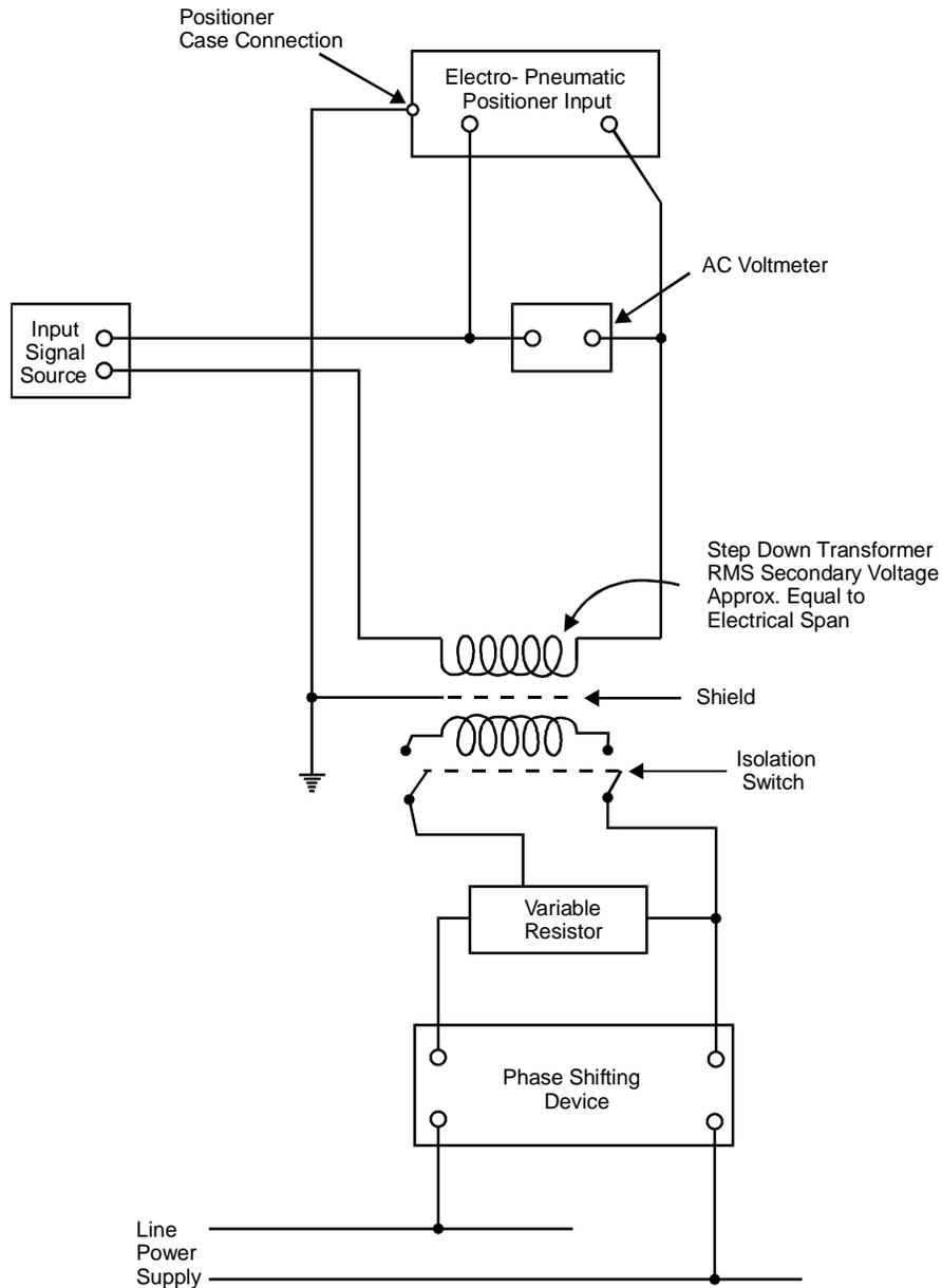
**Figure 6 — Test circuit for normal mode interference influence**
