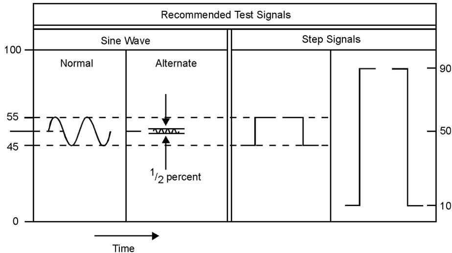
**Figure 15 — Recommended test signals**
