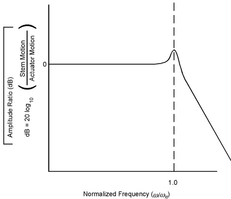
**Figure 4 — Relative stem motion for typical linear actuator**
