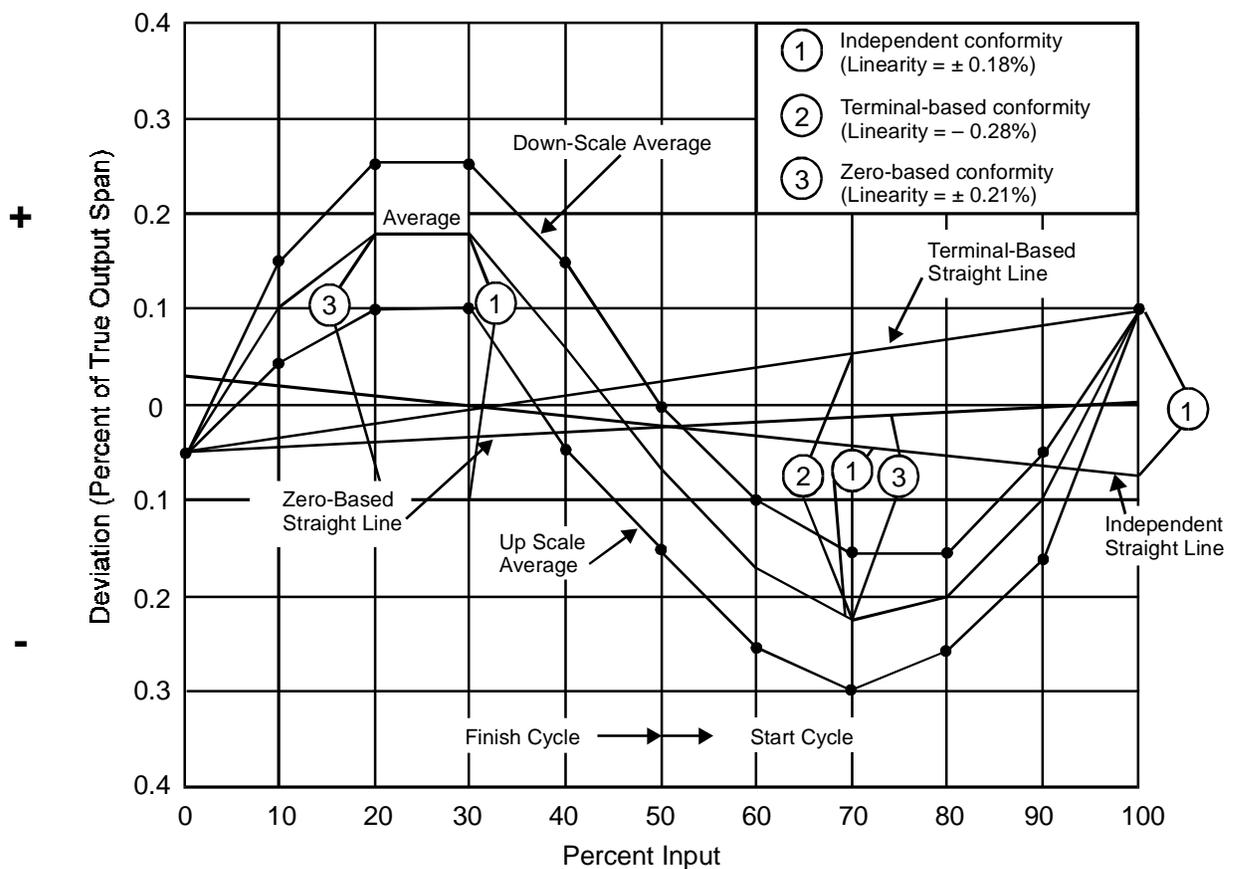
Figure 1 — Calibration curve (of data from Table 1)
