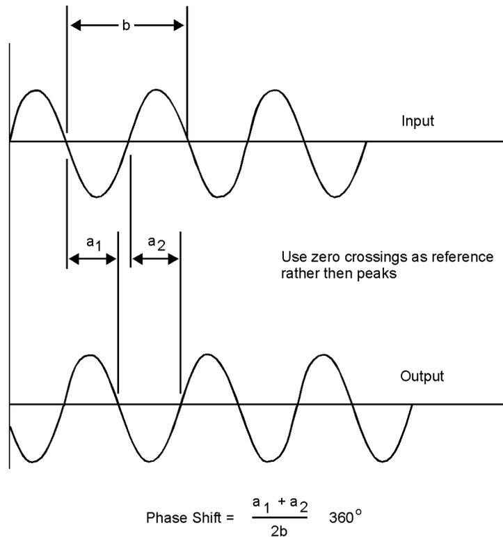
**Figure 17 — Determination of phase shift for distorted output**
