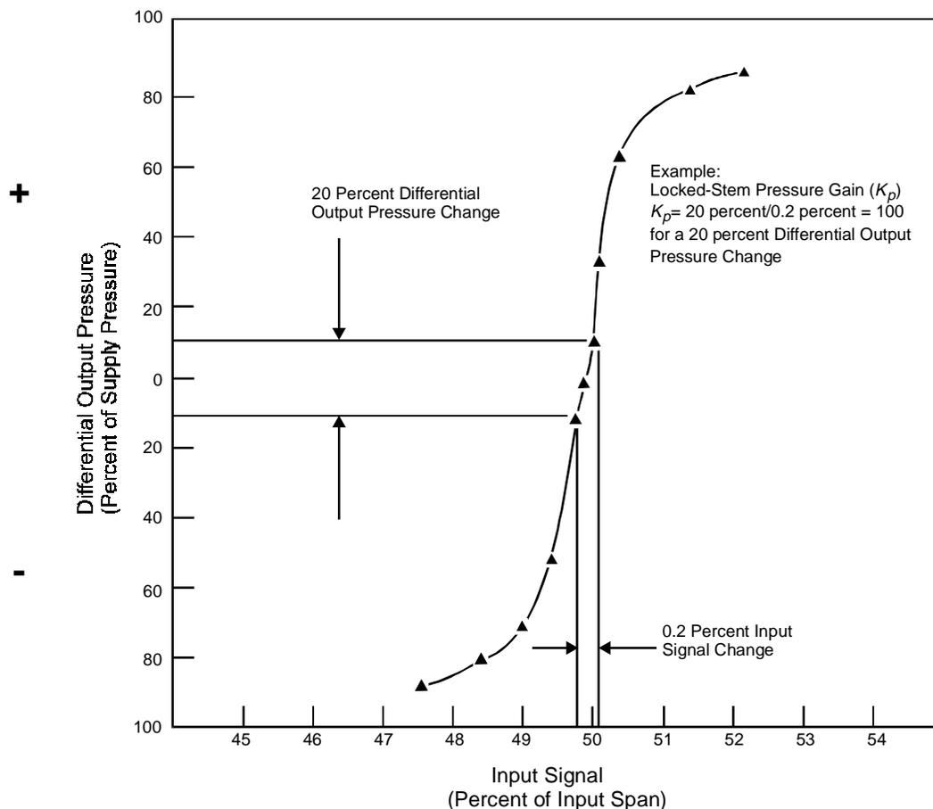
**Figure 11 — Locked-stem pressure gain (double-acting)**
