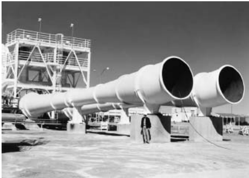
Fig. 33. These two steam jet ejectors serve as part of the pressure recovery system at the U.S. Army's high energy laser system test facility in White Sands, New Mexico. They are each 97 feet long with 96 inch diameter end-suction connections, and are among the largest ever manufactured anywhere. Each ejector handles a large quantity of low molecular weight gas at 120 Torr using the equivalent of 1.044 million pounds of steam per hour at 150 psig during the 14-second cycle.
