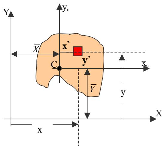
$$I_{xy} = \int xy dA = \int (x + \bar{x})(y + \bar{y}) dA =$$
